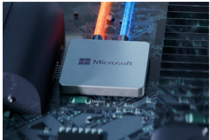
Figure 5: A chip enclosed in casing with coolant pipes within a server blade
